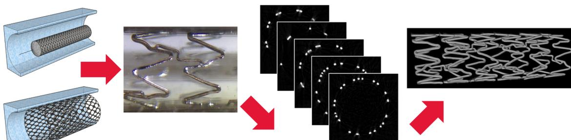
In vitro model fabrication, scanning and in silico reconstruction
