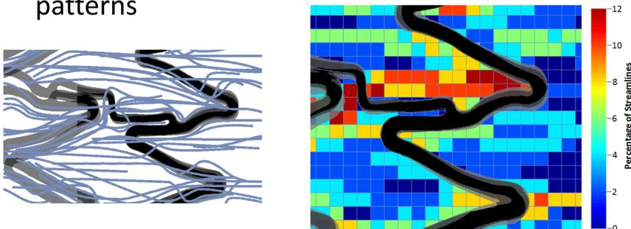
Streamlines and density heat-map of tracked particles
